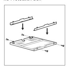
If you use a protection box (an additional accessory), the protective floor directly below the hob is not necessary. The protection box accessory may not be
